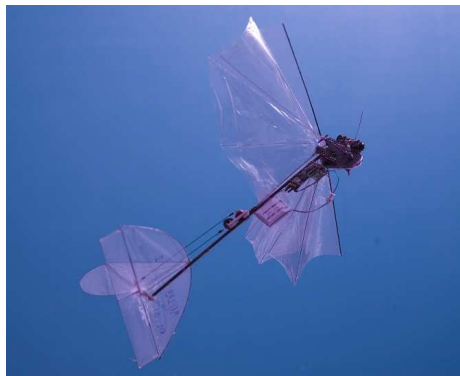
Figure 1: DelFly II has a double pair of flapping wings, driven by a 2 Watt sensorless brushless motor that drives gears with pushrods to the wings. The horizontal stabilizer has an elevator and the vertical stabilizer a rudder. Both are driven by servo's. The flapping frequency is controlled by the power setting of the main motor controller. Onboard electronics comprise of a radio or modem for communication, an autopilot processor with sensors and a special made brushless motor controller.
